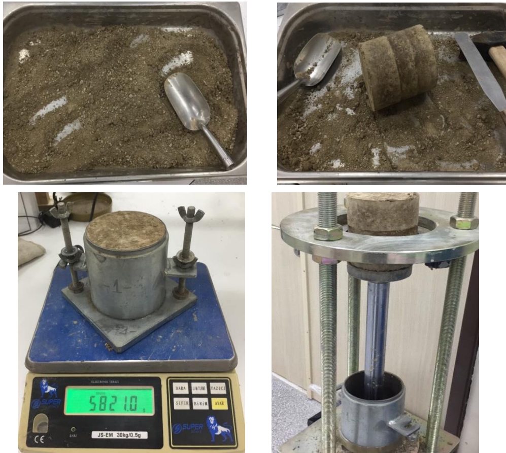
Figure 2. Sample preparation of compaction test
