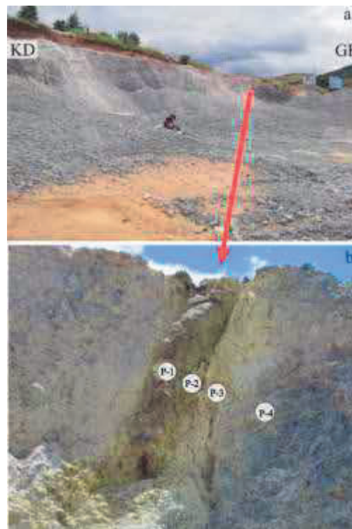
Figure 2 (a) Photo showing general view of the Yukariemirler perlitite deposit, (b) Alteration zone and fault of the Yukariemirler perlitite deposits with sample numbers, and locations.
